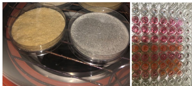
Figure 1. Photograph of the fabricated scaffold samples after freeze drying (left) and when placed in media (right).
