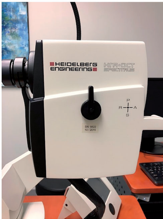
Figure 1. The Heidelberg Spectralis HRA+OCT filter lever wheel includes a polarization filter when in the “P” position. (A color version of this figure is available in the online journal.)
